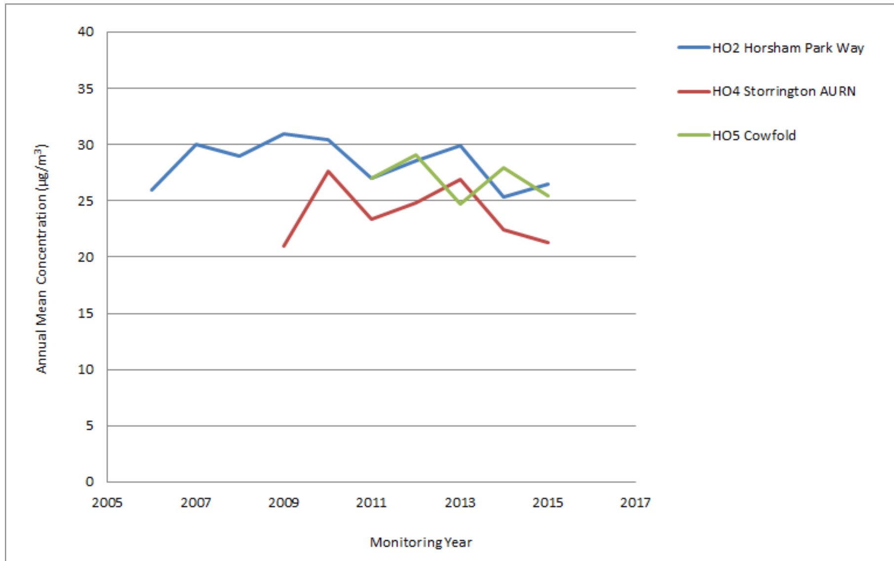
Figure A1 - Trends in Annual Mean NO 2 Concentrations Measured at Automatic Monitoring Sites 2006 - 2015
